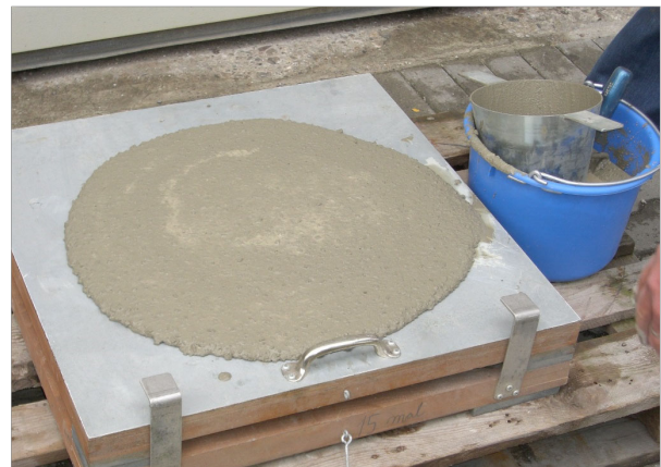
Highly fluid concrete
