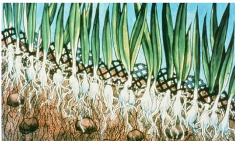
The Geosynthetic reinforces the vegetation root structure...
