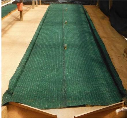
Geosynthetic (unvegetated) erosion control protection installed over test slope
