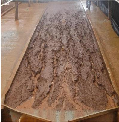
Unprotected Slope after 150 mm/hour rain test event
