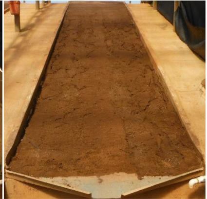
Protected slope (geosynthetic removed) after 150 mm/hour rain test event
