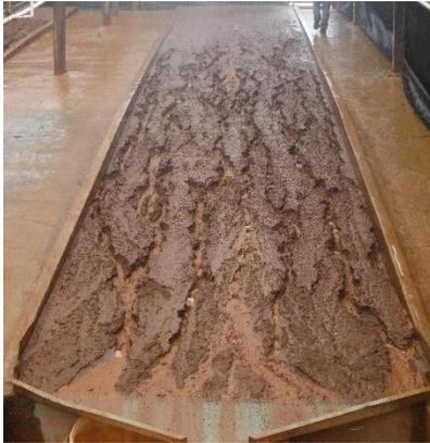
Unprotected Slope after 150 mm/hour rain test event
