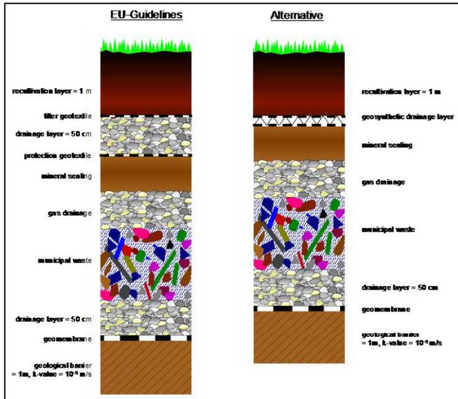
Fig.1: Scheme of the profile of waste landfill site class 2 according to EU guidelines (case 3A, left) and with a drain core as an alternative drainage layer in the cap (case 3B, right)
