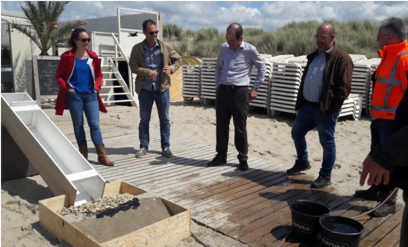
Figure 5. The test set-up with a wave flume and trays with one of the models
