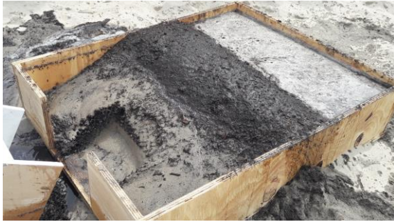
a. Humus in geogrid: slope stayed intact but a lot of overtopping
