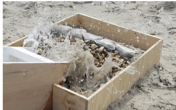
d. Sandbags and gravel
