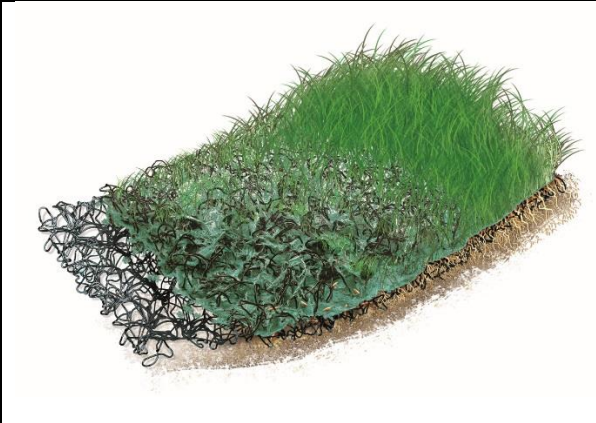
a. Geomat with hydromulching; anchoring with the root system
