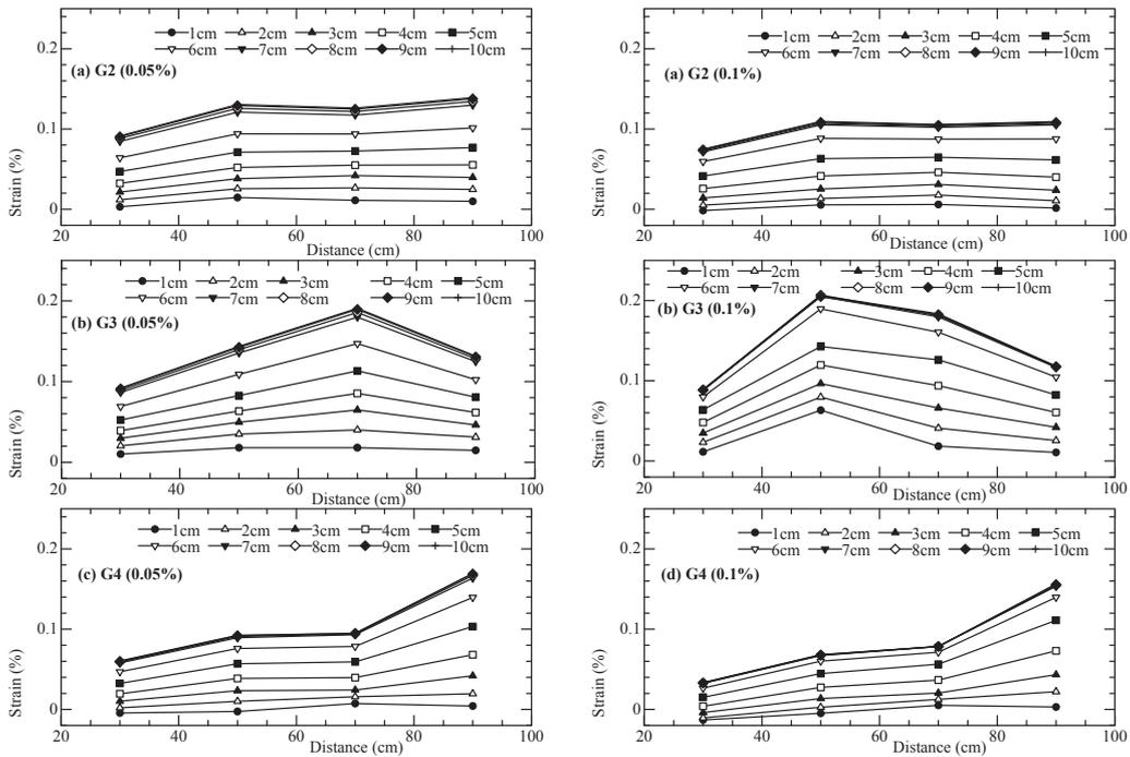
Fig. 9: Strain in geogrids (case 2: 0.016% of prestress)
