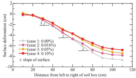
Fig. 6: Surface deformations due to settlement of 10cm.
