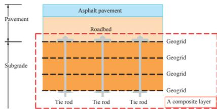
**Fig. 1:** Confined-reinforced subgrade (Kuwano et al., 2013)
