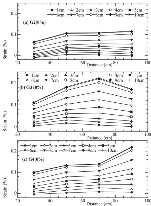
Fig. 7: Strain in geogrids (case 1: 0.0% of prestrain).
