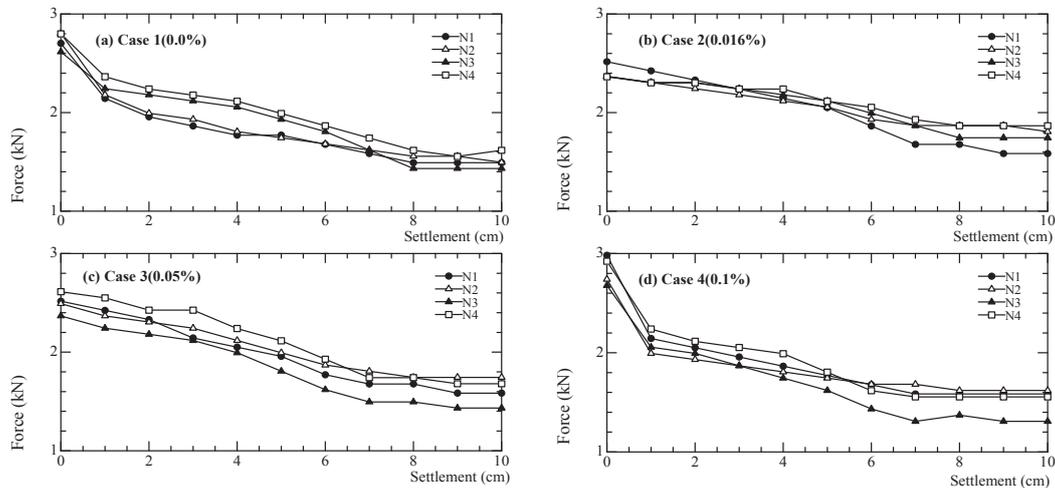
Fig. 12: Force in tie-rods: (a): Case 1-0%, (b) case 2-0.016%; (c) case 3-0.05% & (d) case 4-0.1%.
