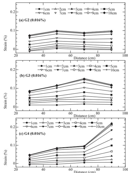
Fig. 8: Strain in geogrids (case 2: 0.016% of prestrain)
