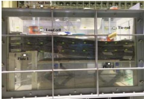
Fig. 5: Deformation of CRE due to settlement
