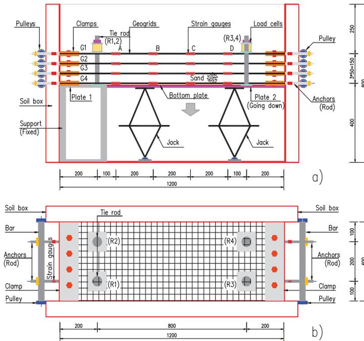
Fig. 4: Experimental model, (a): elevation view, (b): plan view
