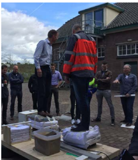
Figure 2. The piled embankment models after loading with shaking and a surcharge load
