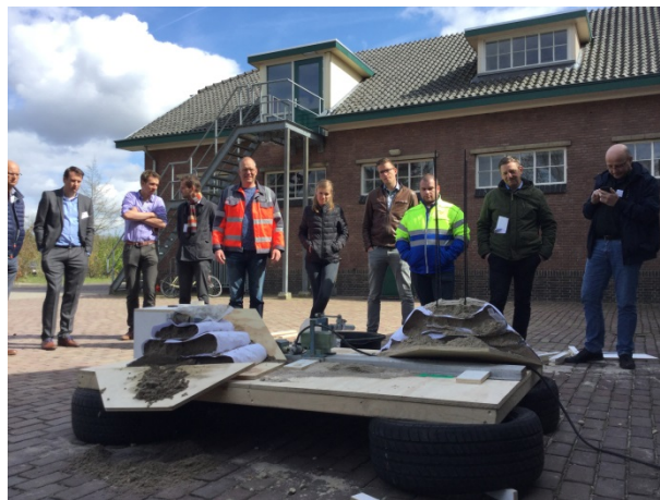
Figure 4. Both embankments with 45 degrees slopes were earthquake resistant. Removing their supporting box walls helped: the models were destroyed on the shaking table.
