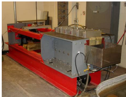
Figure 1. Dynamic direct shear machine for geosynthetic clay liners (Fox et al. 2006).
