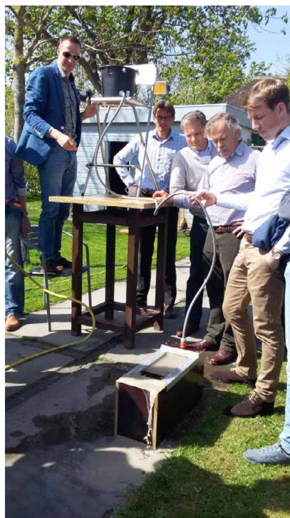
Figure 2 There's water in the bucket that has been connected to the model. Because of this, there is a gradient of about 2 metres under de 'levee'. That 'levee' is composed of a glass plate, possibly with anti-piping features. The development of piping is visible through the glass plate.
