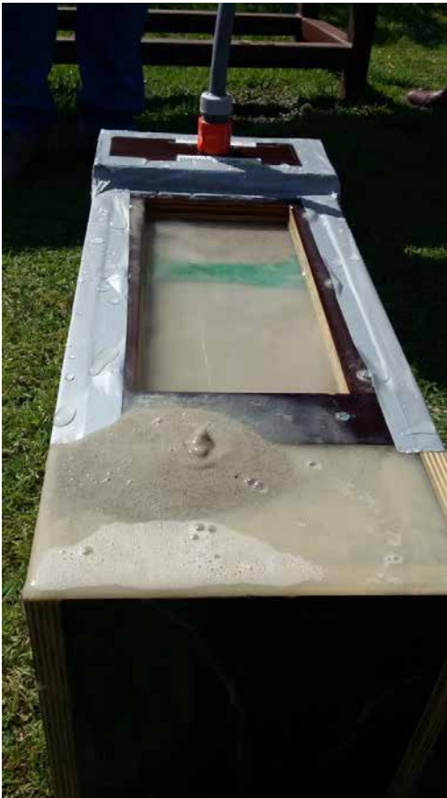
Figure 3 Sand boil that takes along sand. Beneath the glass, you can see the green-coloured “geotextile” beneath the middle of the levee. On the right: NGO-euros.
